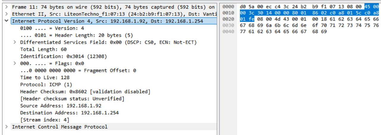
Frame 11: 74 bytes on wire (592 bits), 74 bytes captured (592 bits) on
