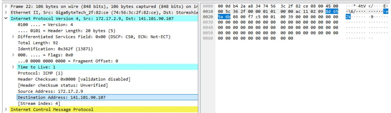
Frame 22: 106 bytes on wire (848 bits), 106 bytes captured (848 bits) on interface **Ethernet II, Src: GigaByteTech\_2f:82:ce (74:56:3c:2f:82:ce)**, Dst: Stormshield (141.101.90.107)
